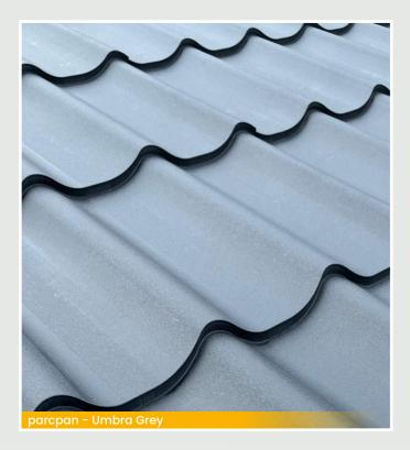
Parcpan is a tile-effect roof sheet meticulously designed to parallel the charm of traditional pan tiles. Crafted from premium-grade Aluzinc steel and coated with a durable 35-micron wrinkle effect polyester coating, Parcpan provides an attractive, lightweight, and cost-effective roofing solution. Perfectly suited for holiday homes, Parcpan delivers both style and durability, making it an ideal choice for the industry.
